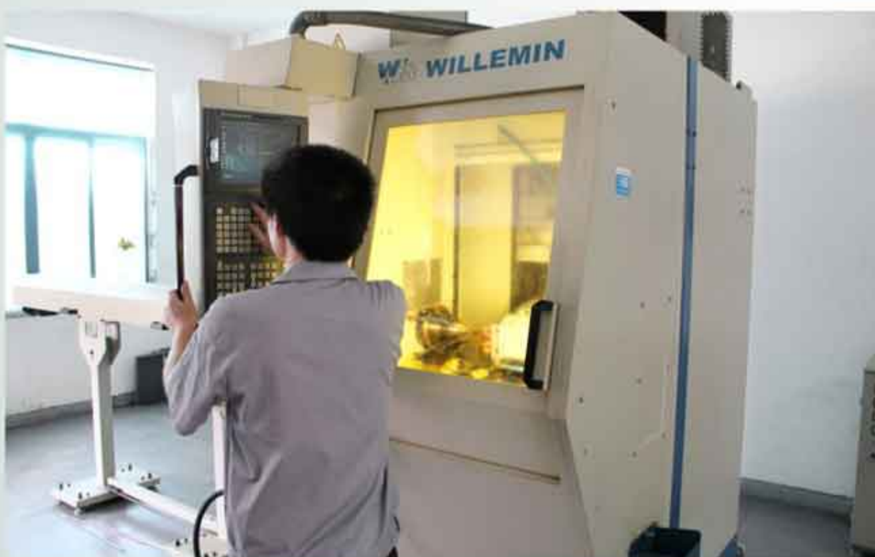
瑞士威力铭马科戴尔五轴联动数控加工中心加工内窥镜及手术钳精密零件 5Axes CNC Machine made in WILLEMIN-MACODEL S.A./Switzerland for high precision mechanical parts production
