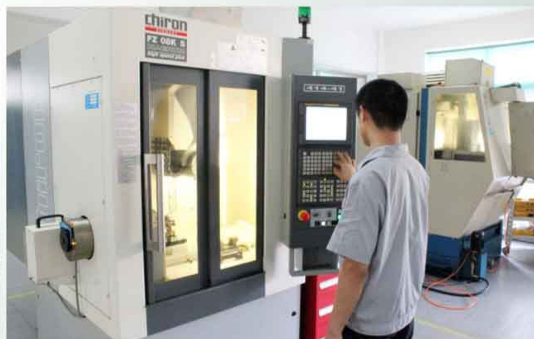
德国巨浪 (Chiron) 复合加工中心实现高速、高效、高精度柔性加工 Compound CNC machine from Chiron Germany for fast, efficient and high precision production in wide range of flexibility
